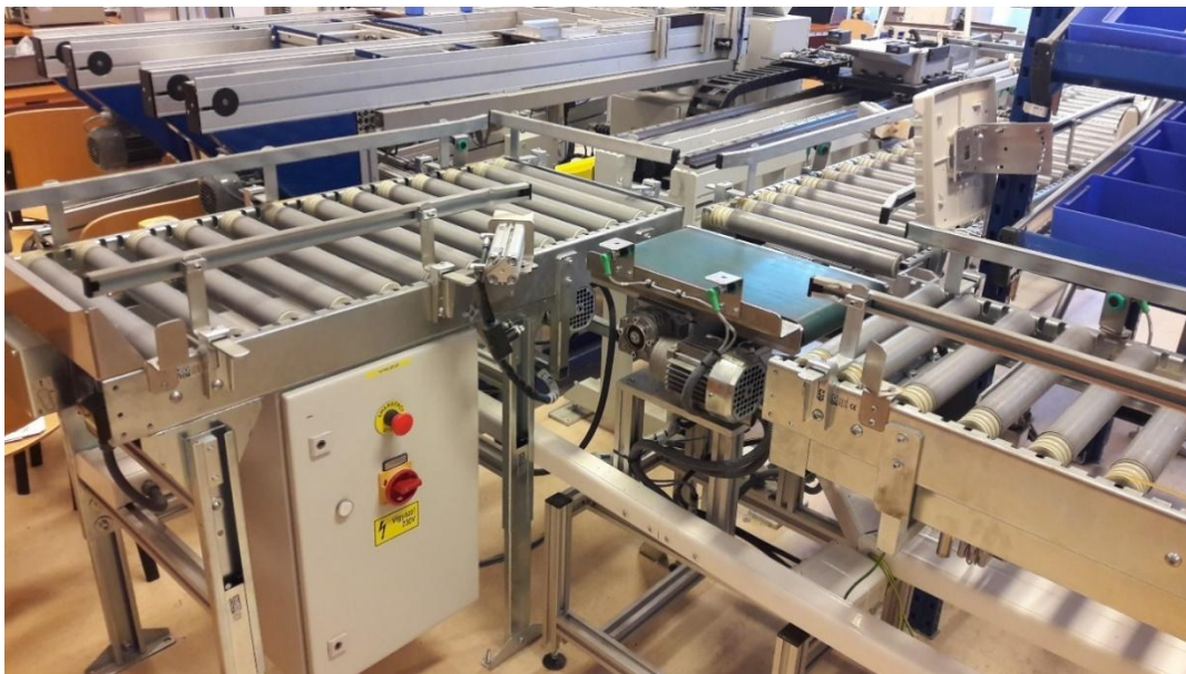
Figure 4. A turning table with a pneumatic gripper on the left and an RFID reader on the right (Source: created by the authors)
