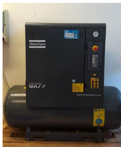
Figure 3. The compressor that provides the pressurized air for the operation of the roller conveyor track (Source: created by the authors)
