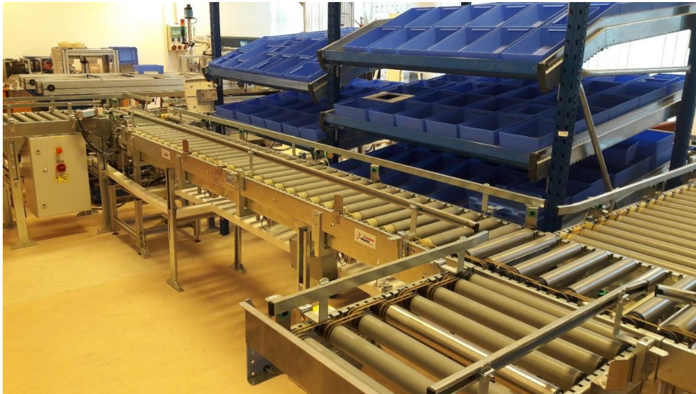
Figure 2. A section of the rolling conveyor track with the manual tilted stand in the middle (Source: created by the authors)
