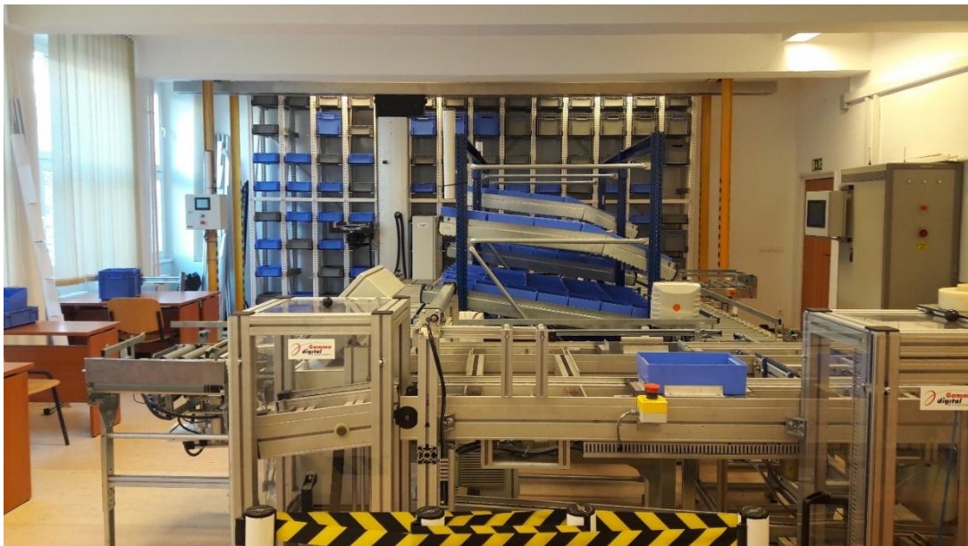
Figure 6. The palettizing station in the foreground, together with the previously described systems in the background (Source: created by the authors)
