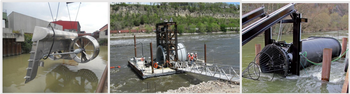
Figure 2 - different solutions of hydrokinetic turbines - Twin-Turbine [4] (left), Hydro Green Energy [6] (center) and KSB AG [3] (right)
