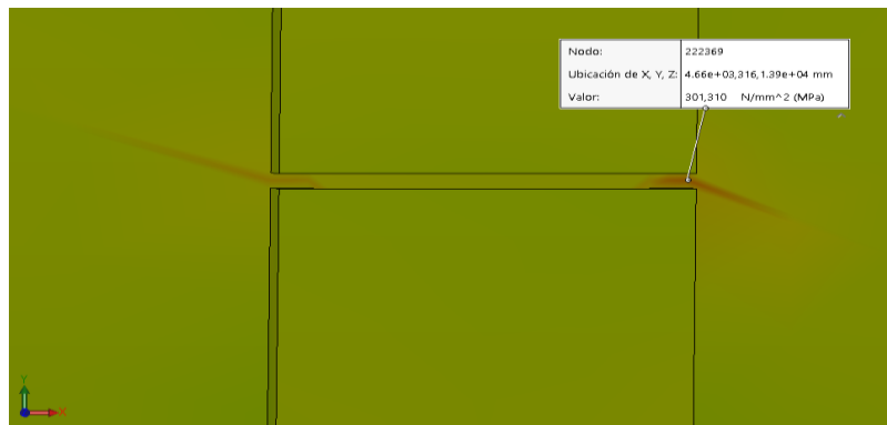
Figure 3.8 Normal stresses on the Y axis in the failure zone. Source: (author).
