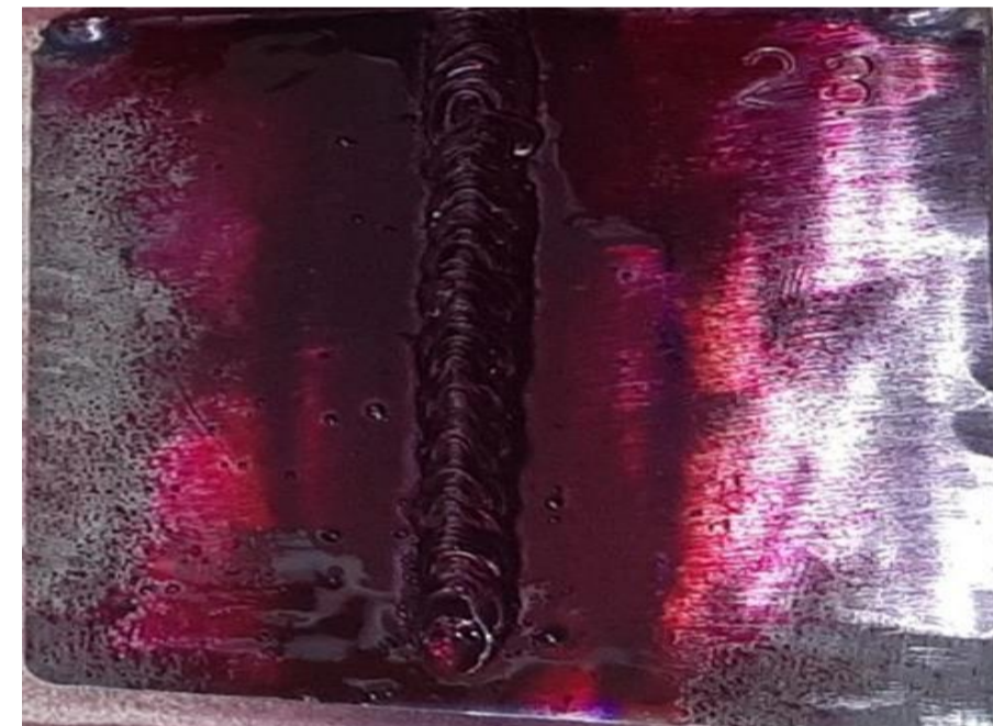
Figure 2. Non-destructive liquid penetrant test
