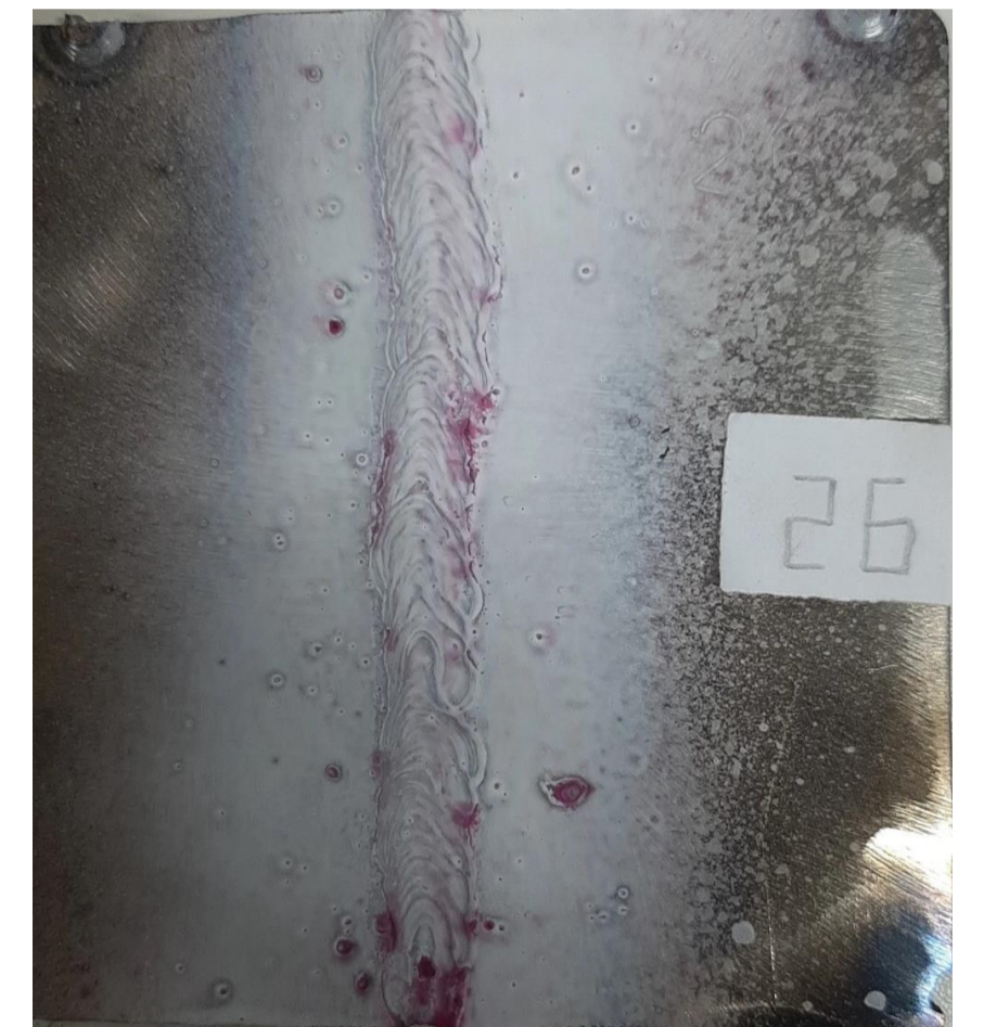
Figure 4. Application of penetrating post-liquid developer
