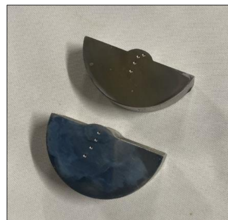
Figure 3. Hardness test (Own elaboration).
