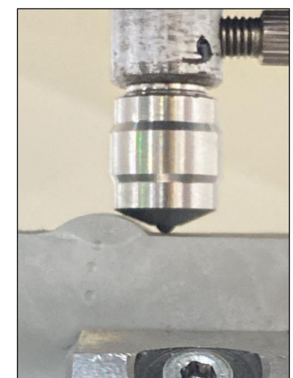
Figure 4. Vertical hardness test (Own elaboration).
